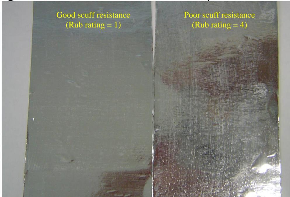
It was found that scuff resistance is primarily a function of the coating chemistry, as well as the EB dosage applied to the coating. A more reactive chemistry and a higher EB dosage are correlated with better scuff resistance, as increased levels of cross-linking tend to improve the abrasion resistance of the coating. Coatings with a lower inherent surface energy also lead to improved scuff resistance.
